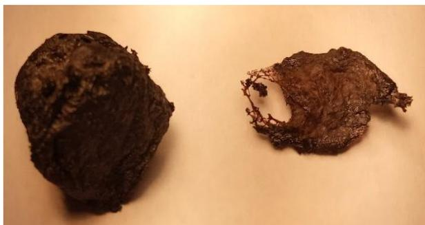
**Figure 19.** The amorphous thick layer of the char after the reaction of APP and PER (left) and the outer thin rigid layer of the char after the reaction of APP and MEL (right) at the temperature 600 °C.
