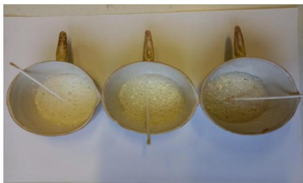
Figure 3. Appearance of adducts after exposure at 100° C for 5 hours.
