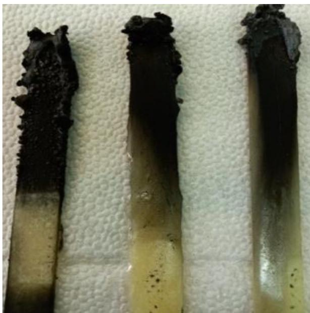
**Figure 14.** Appearance of samples after testing according to UL 94 standard: from left to right - EPG-32; EPG-36; EPG-37.
